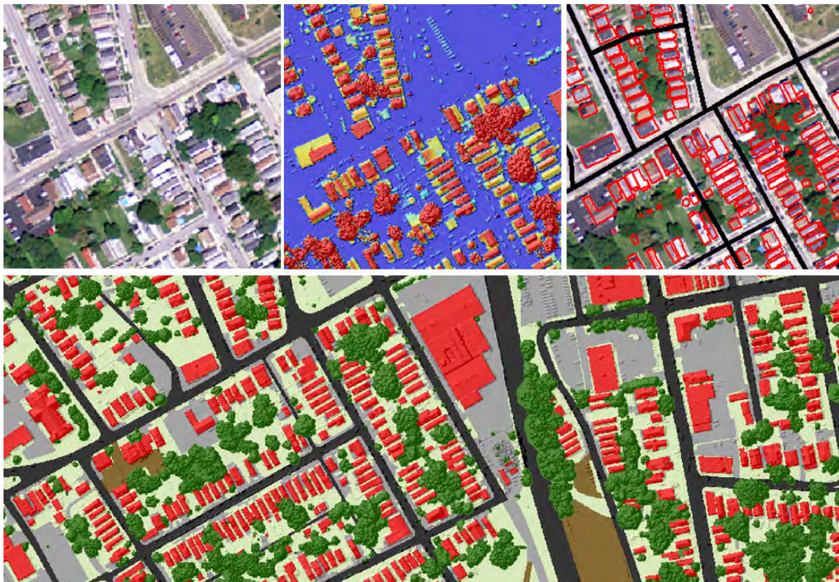
Figure 4. Aerial images, LiDAR, and ancillary map data are used to create detailed land cover maps.
