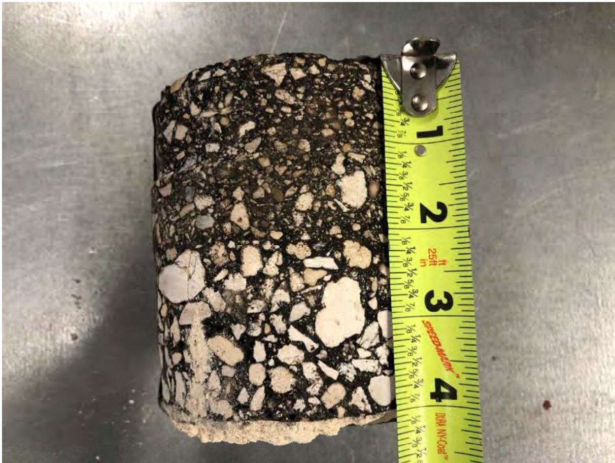
Core C-04: 4" Asphalt 10" Limerock Base SAND with silt (A-3) Subbase
