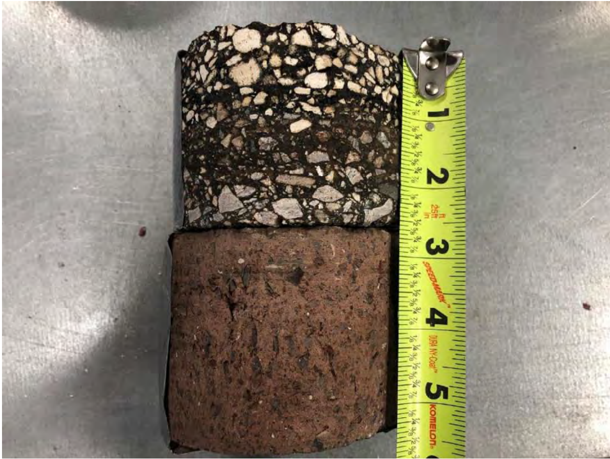
Core C-02: 2 ½" Asphalt 2 ¾" Paver No Base Encountered SAND with silt (A-3) Subbase
