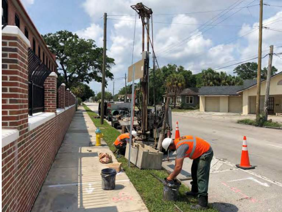
Figure 3: Performing SPT-01 on N. Howard Ave. (photographed June 6, 2018)
