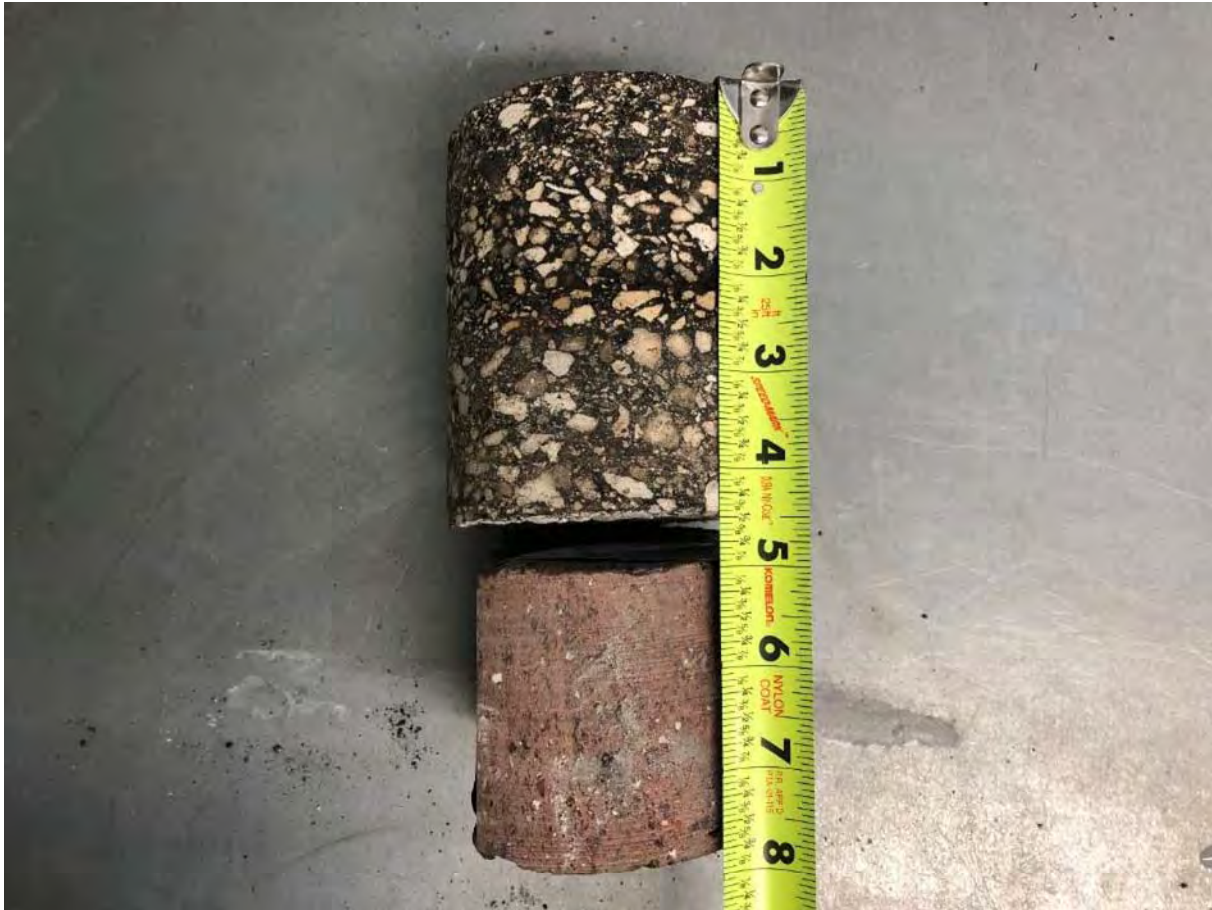
Core C-01: 4 ½" Asphalt 3" Paver 4 ½" Shell Base SAND with silt (A-3) Subbase
