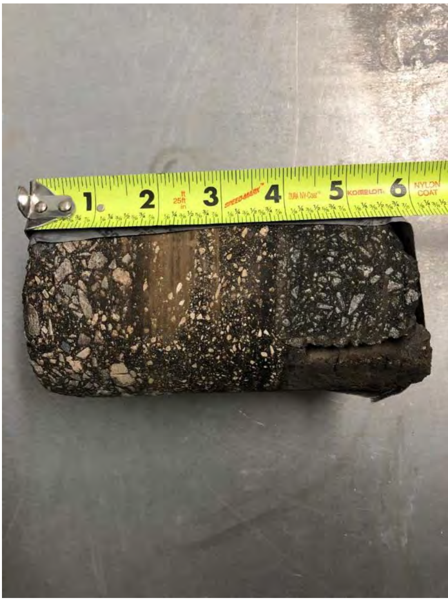
Core C-10: 6" Asphalt (saw cut captured in bottom layer as shown) No Base Encountered SAND with silt (A-3) Subbase
