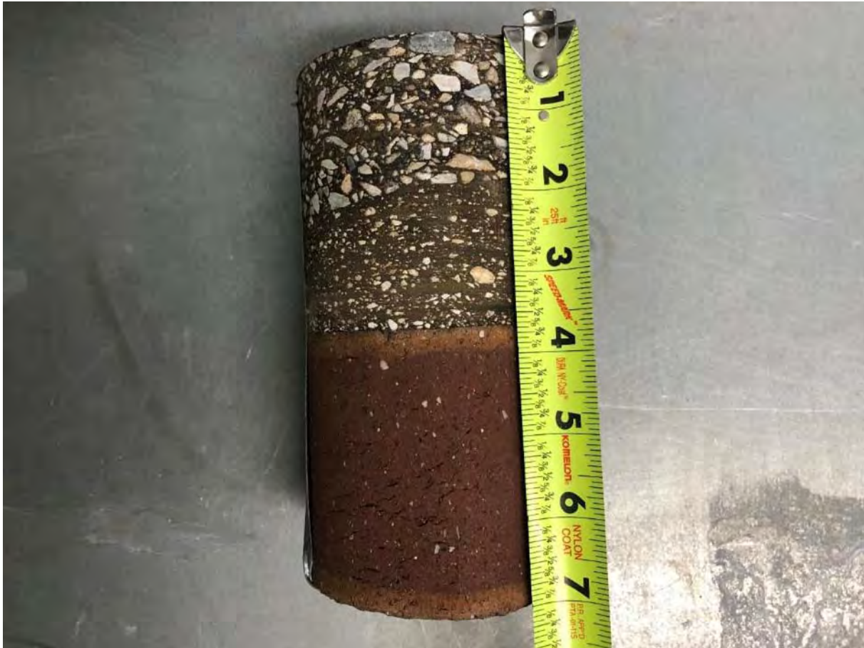
Core C-09: 3 ½" Asphalt 3 ½" Paver No Base Encountered SAND with silt (A-3) Subbase
