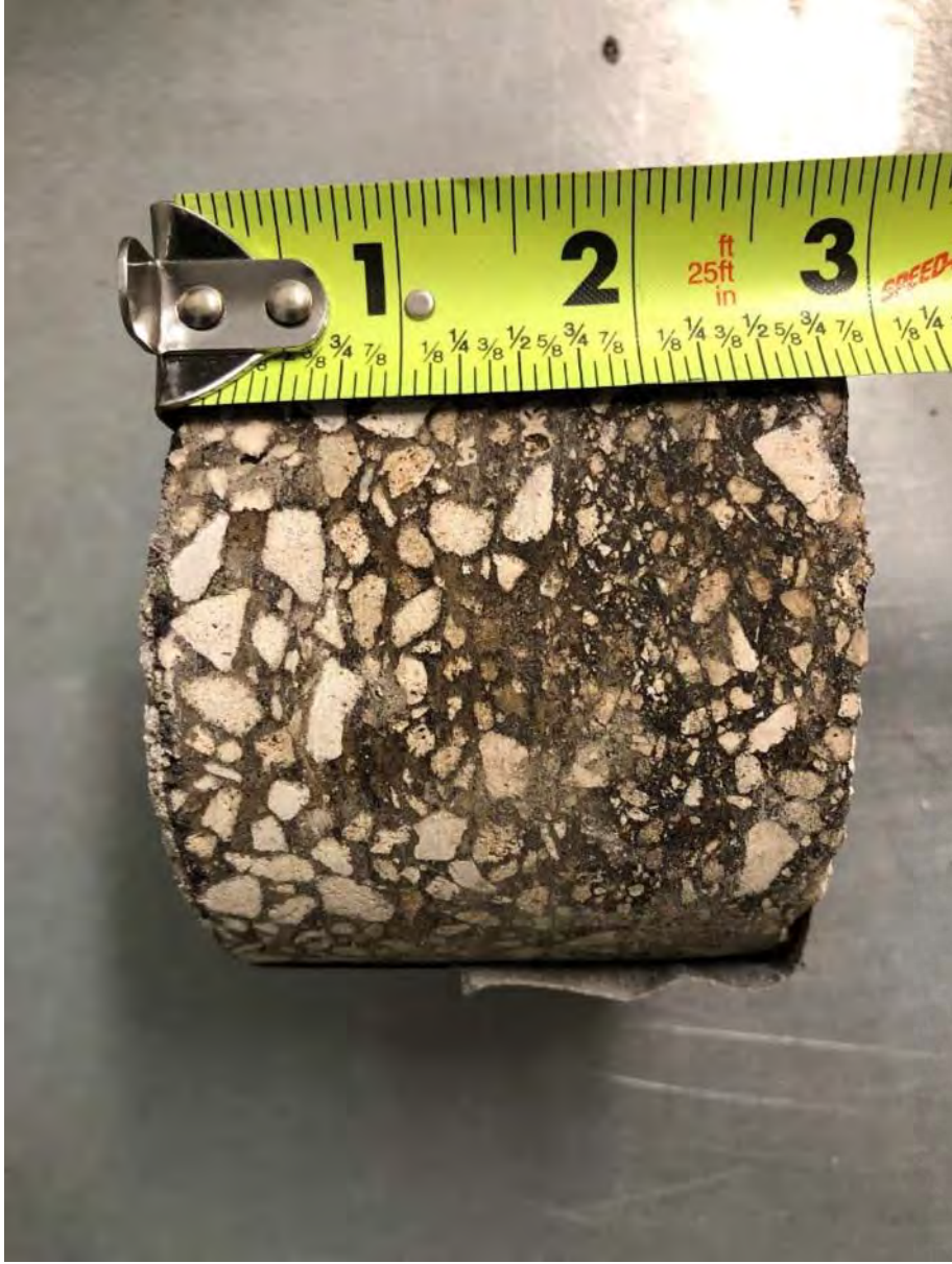
Core C-06: 2 ¾" Asphalt 9 ¼" Limerock Base SAND with silt (A-3) Subbase
