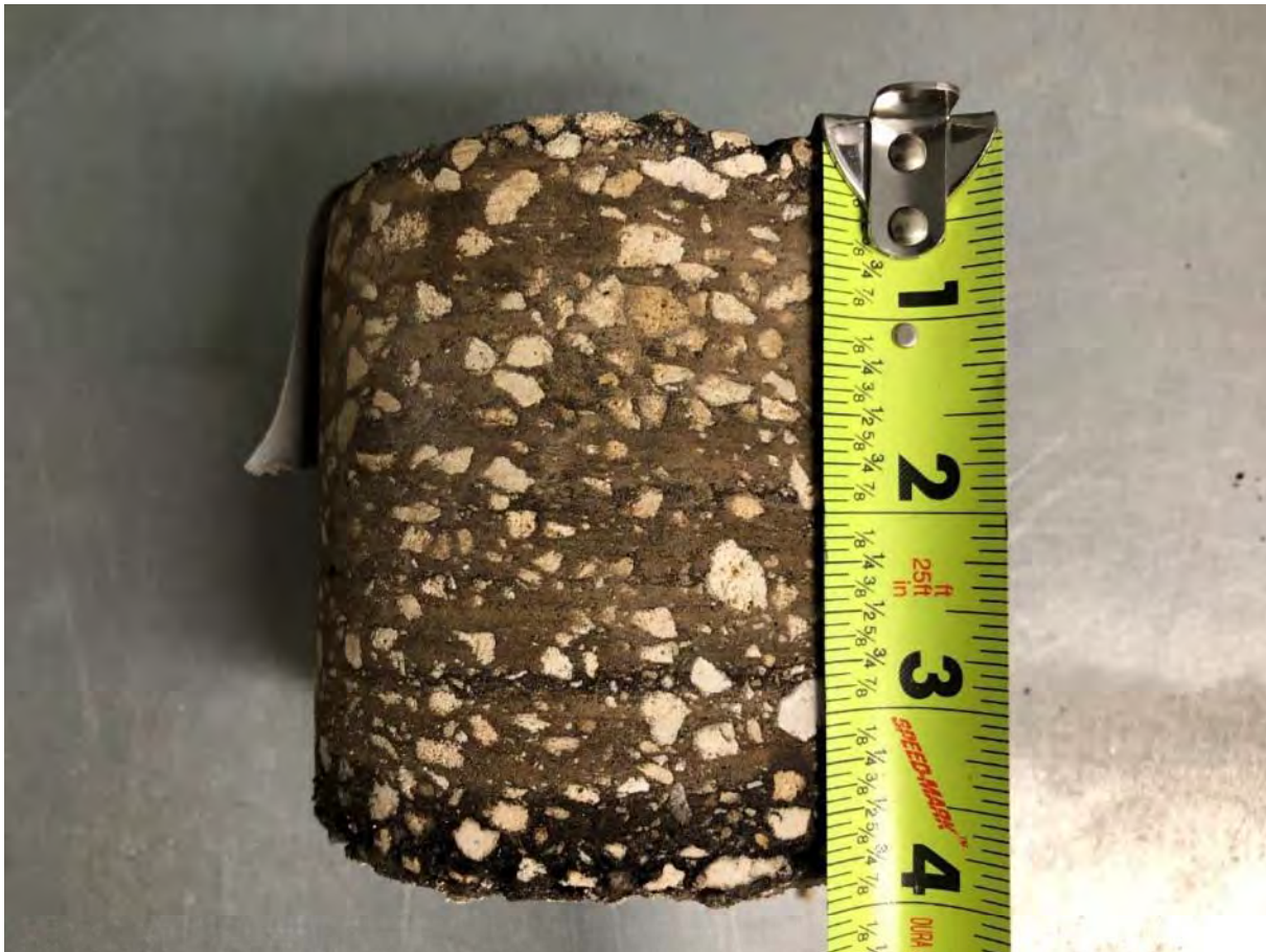
Core C-07: 3 3/4" Asphalt 11" Limerock Base SAND with silt (A-3) Subbase
