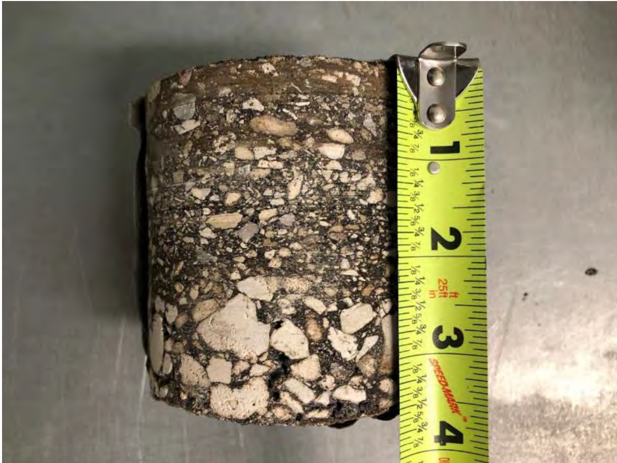
Core C-05: 3 ½" Asphalt 8 ½" Limerock Base SAND with silt (A-3) Subbase
