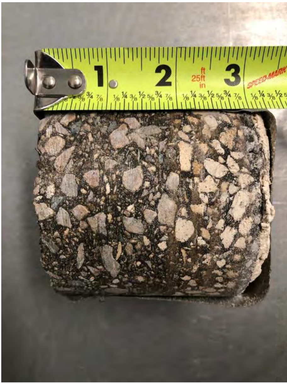
Core C-08: 3" Asphalt 11" Limerock Base SAND with silt (A-3) Subbase
