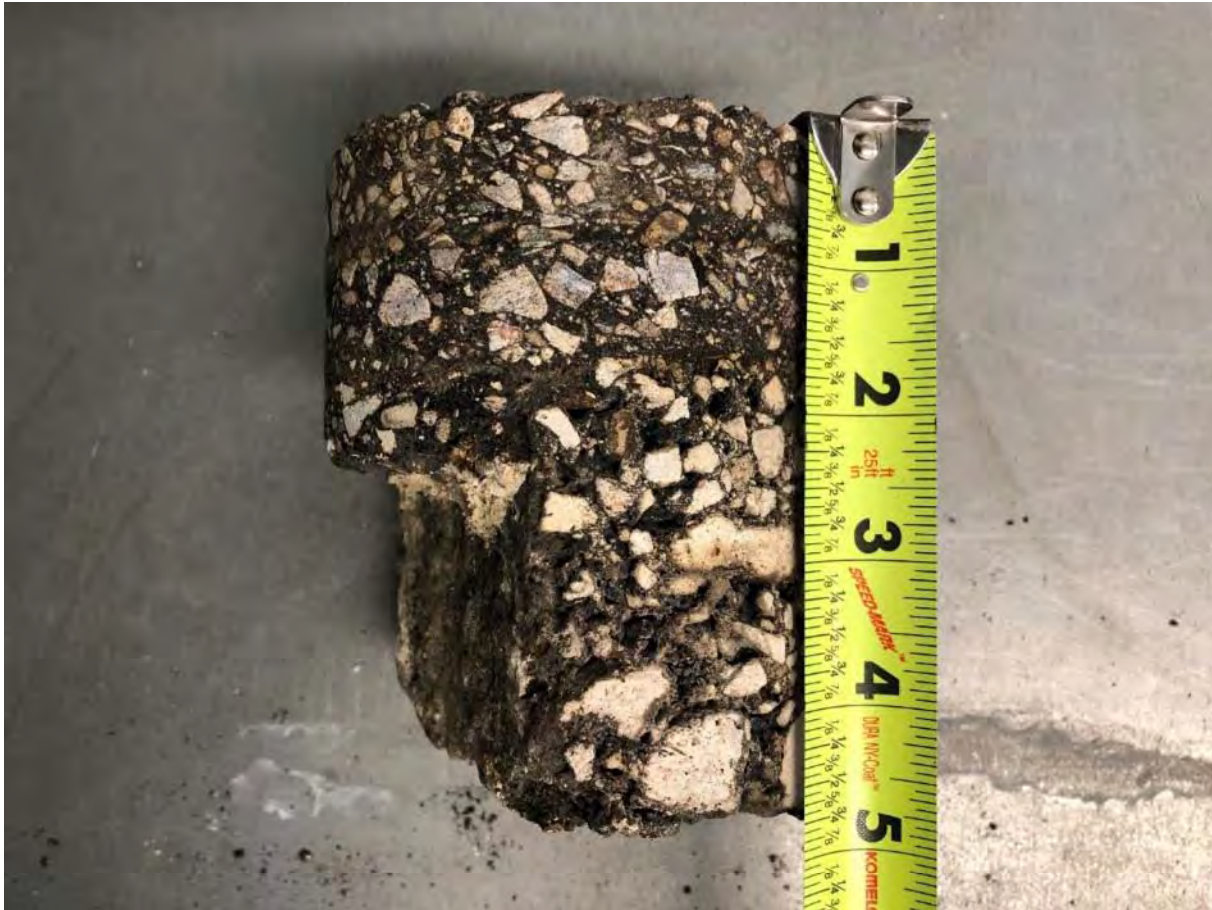
Core C-03: 4 ¾" Asphalt (cracked underneath as shown) 7 ¼" Limerock Base SAND with silt (A-3) Subbase
