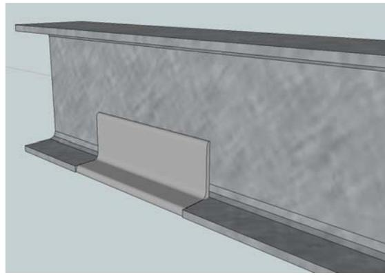
**Figure 4:** Typical Web and Flange Repair
