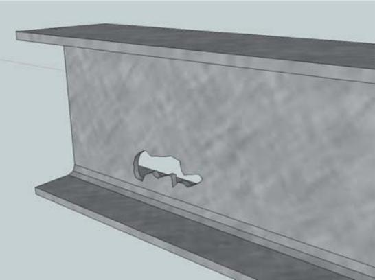
**Figure 5:** Typical Stringer Prior to Repair
