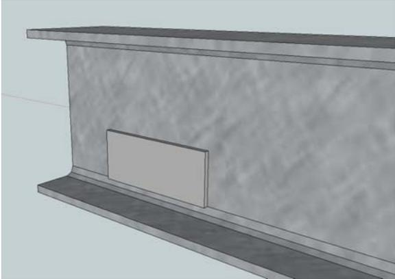
**Figure 6:** Typical Stringer Web Repair
