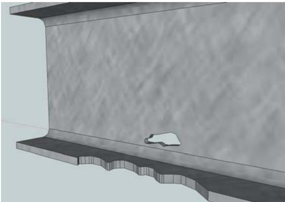
**Figure 3:** Typical Stringer Prior to Repair
