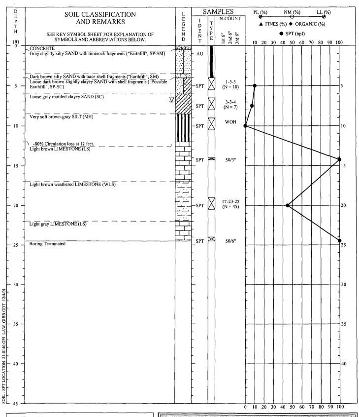
DRILLER: EQUIPMENT: CME Power Drill Rig METHOD: Rotary Wash with Bentonite "Mud", ASTM D-1586 HOLE DIA.: 2 15/16 inches REMARKS:
