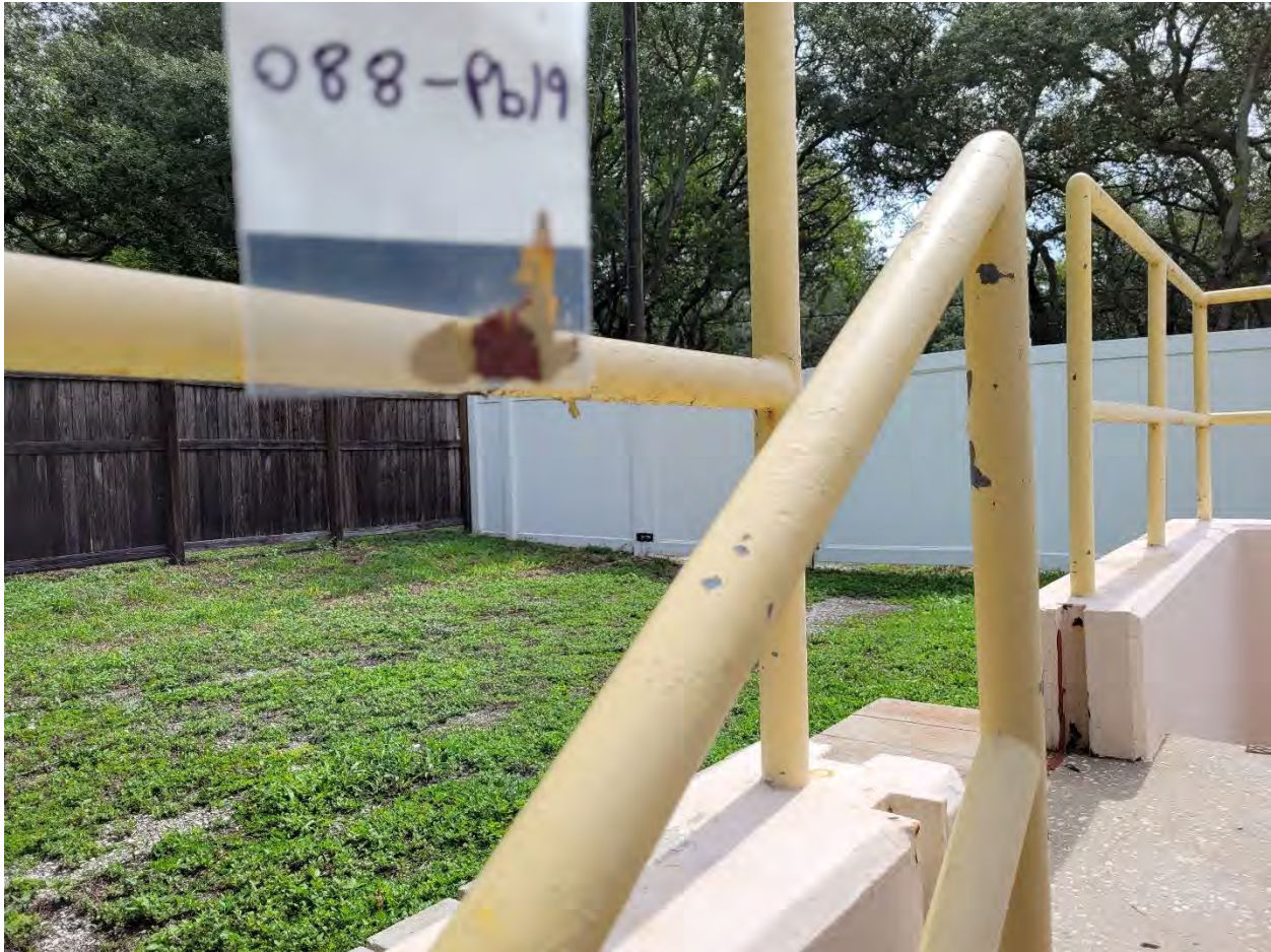
088-PB 19: Yellow Paint on Metal Rails [0.59 % wt]
