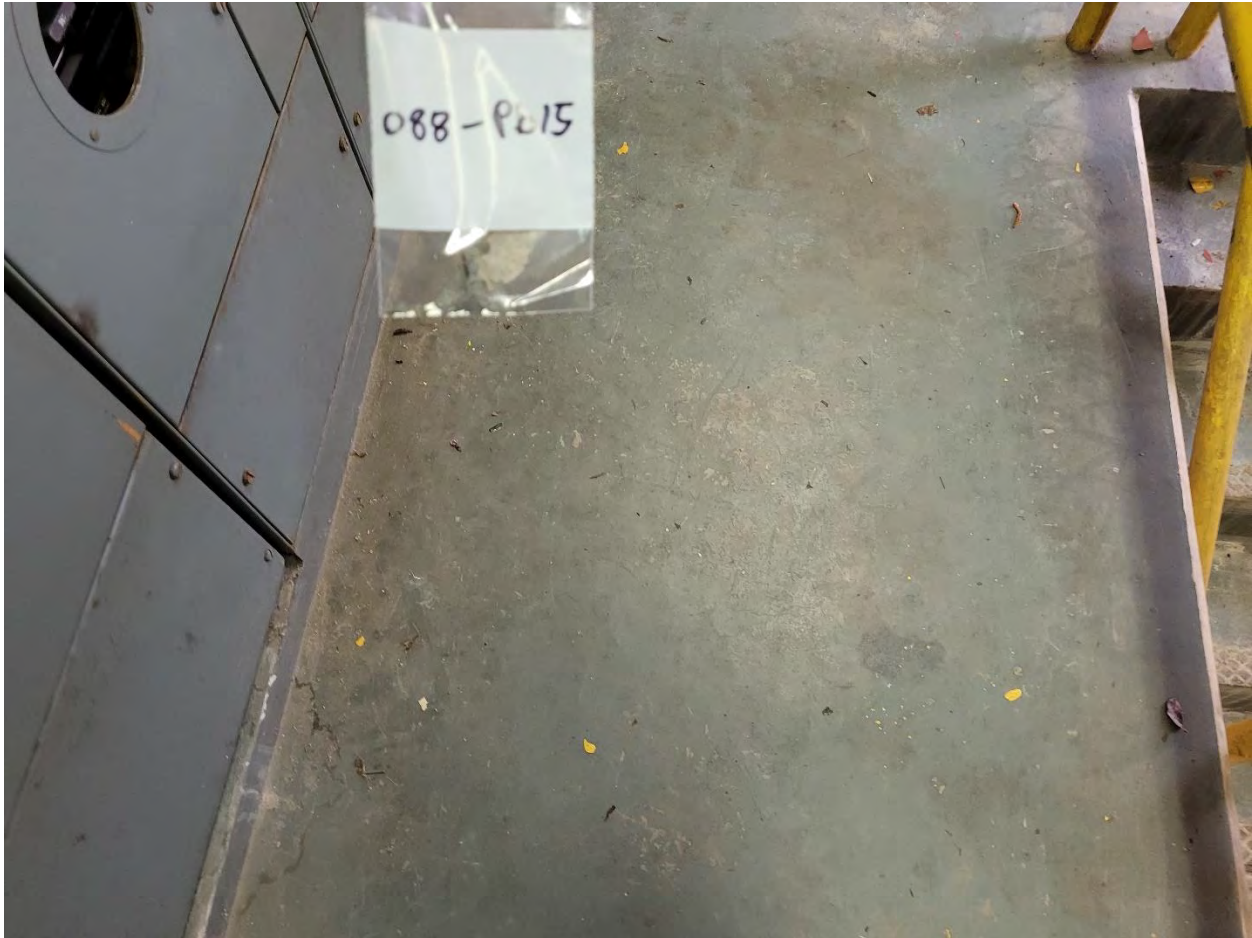
088-PB 15: Grey Paint on Concrete Floor [0.021 % wt]
