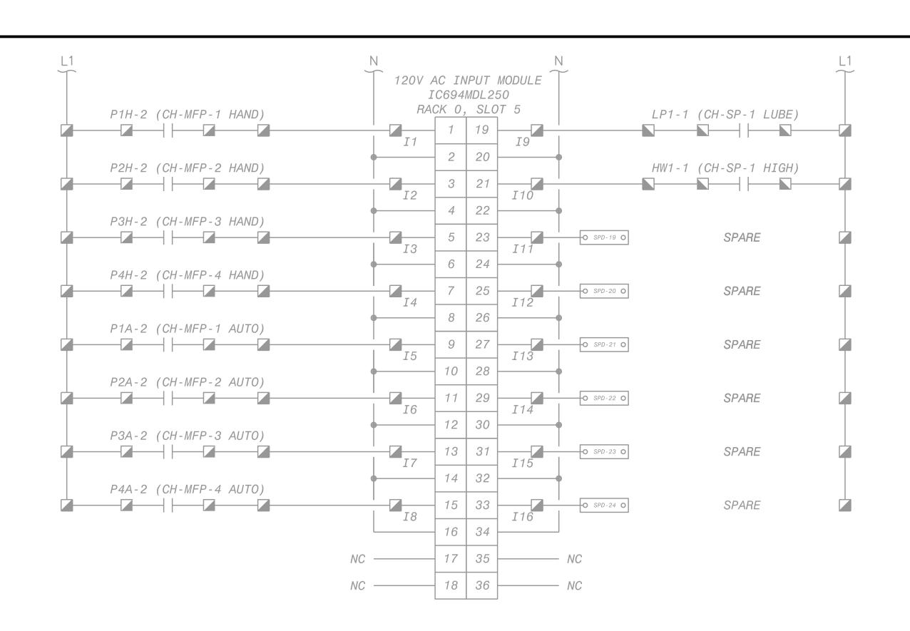
PLC DISCRETE INPUT CARD WIRING DIAGRAM - SLOT 5
