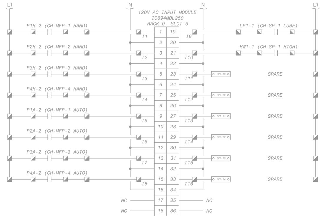
PLC DISCRETE INPUT CARD WIRING DIAGRAM - SLOT 5
