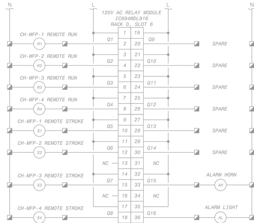
PLC RELAY OUTPUT CARD WIRING DIAGRAM - SLOT 6
