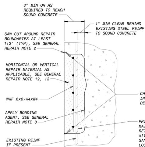
**TYPE III - HORIZONTAL, VERTICAL, OR OVERHEAD CONCRETE SURFACE REPAIR WITH NO DAMAGE TO EXISTING REINFORCING STEEL**
