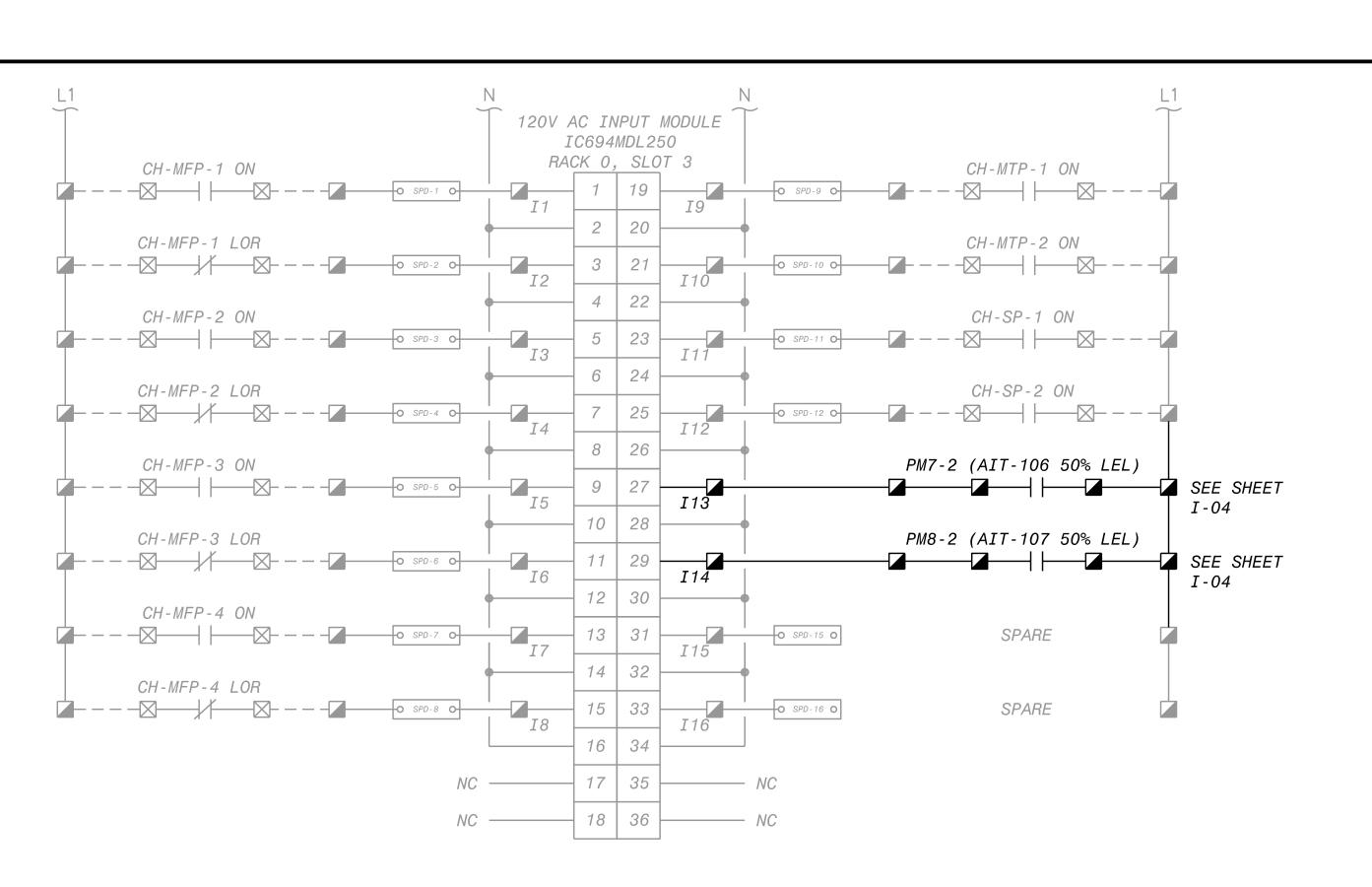
PLC DISCRETE INPUT CARD WIRING DIAGRAM - SLOT 3
