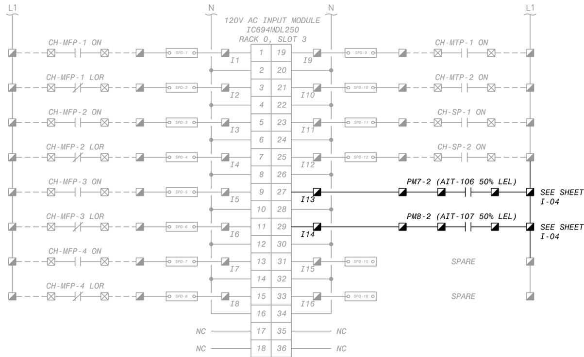
PLC DISCRETE INPUT CARD WIRING DIAGRAM - SLOT 3
