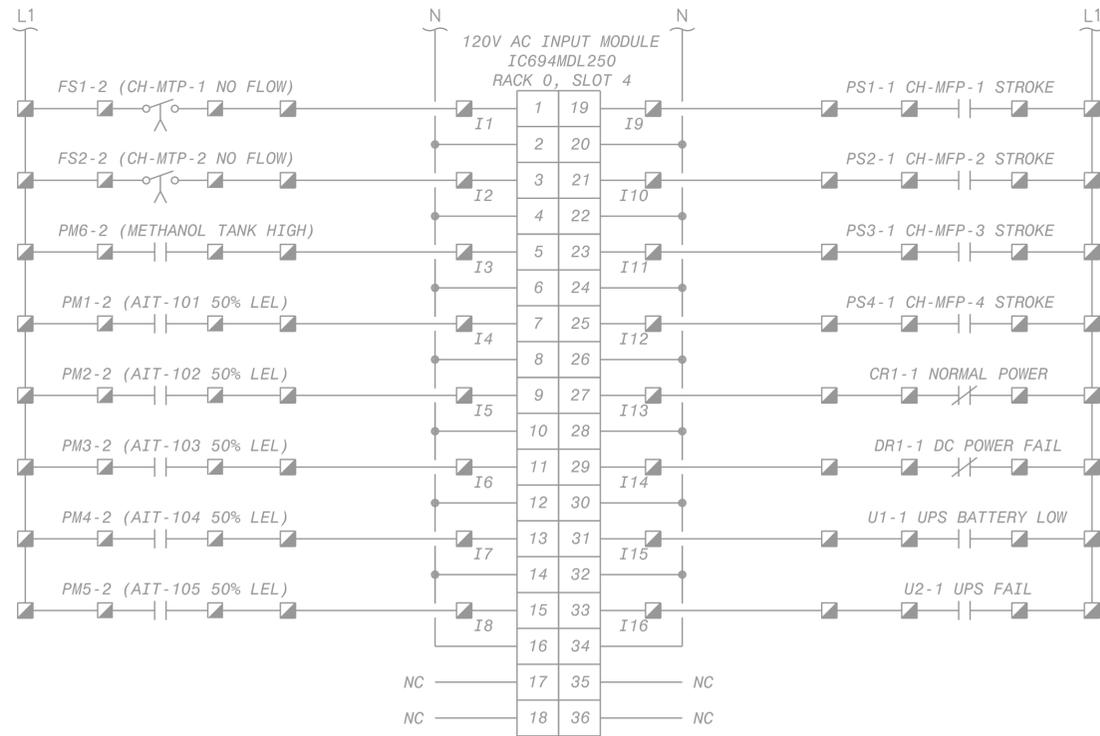
PLC DISCRETE INPUT CARD WIRING DIAGRAM - SLOT 4
