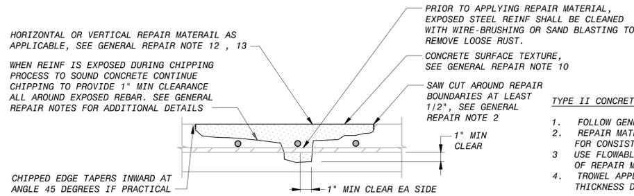
**TYPE II - HORIZONTAL, VERTICAL, OR OVERHEAD CONCRETE SURFACE REPAIR**
