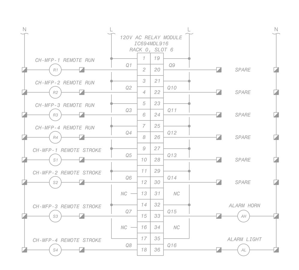
PLC RELAY OUTPUT CARD WIRING DIAGRAM - SLOT 6
