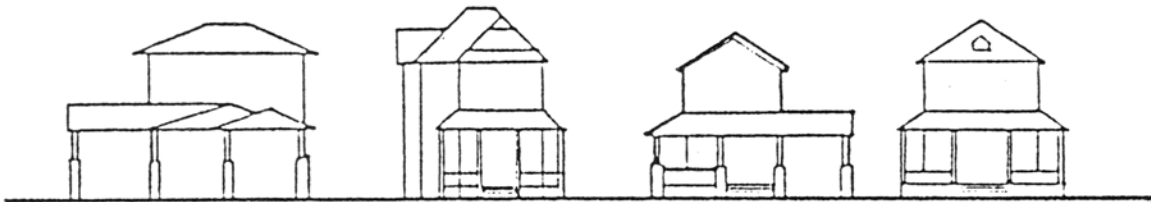
Appropriate: height and width consistent with neighboring houses.
