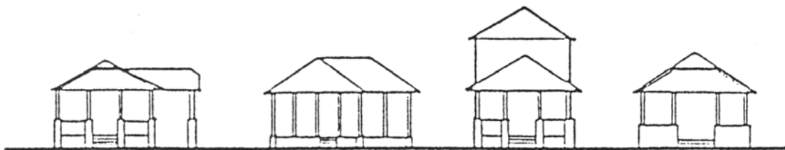
Appropriate: porch and hipped roof break down height and mass of building.
