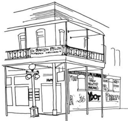
Flat signs can be attached to building fronts. These should be flush-mounted
