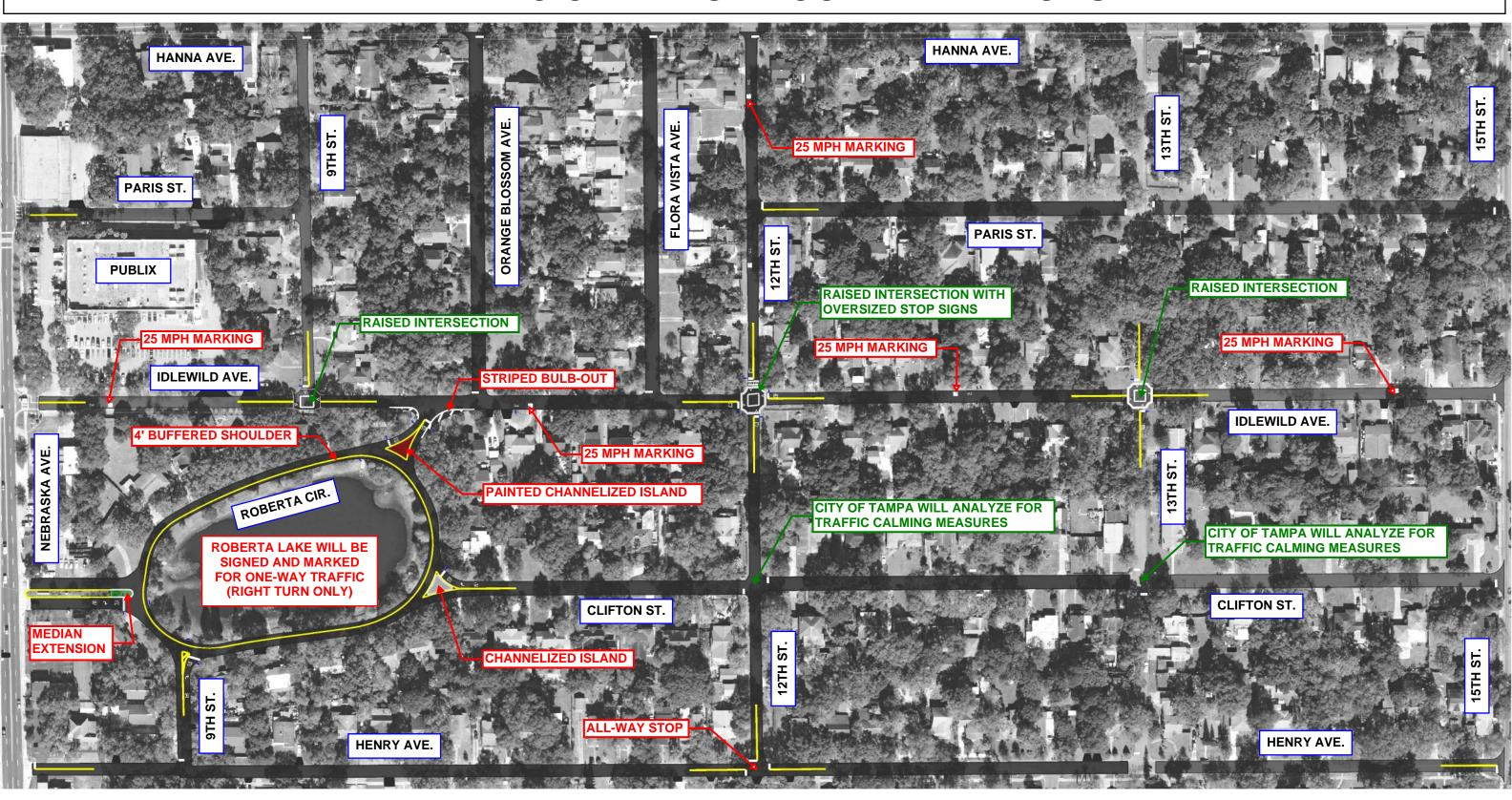
NEW STOP BARS AND PAVEMENT STOP MESSAGES WILL BE ADDED TO ALL EXISTING STOP SIGN LOCATIONS
