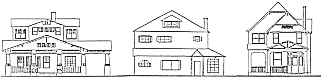
Inappropriate: Doors and windows are spaced awkwardly and window style is out of character with neighborhood.
