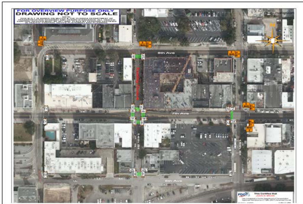
Maintenance of Traffic (MOT) Plan sample
