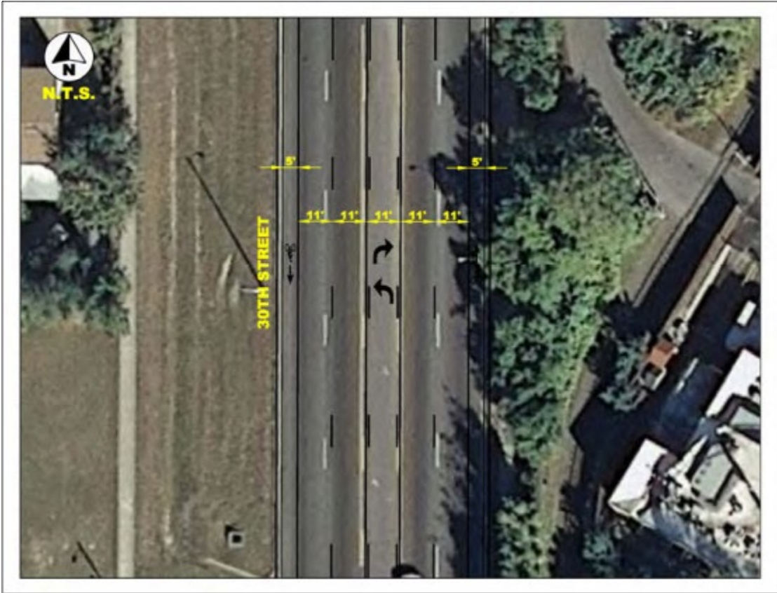
Aerial of the proposed lane improvements, north of Busch Boulevard, displaying reduced 11' vehicle lane widths plus 5' on-road bicycle lanes.
