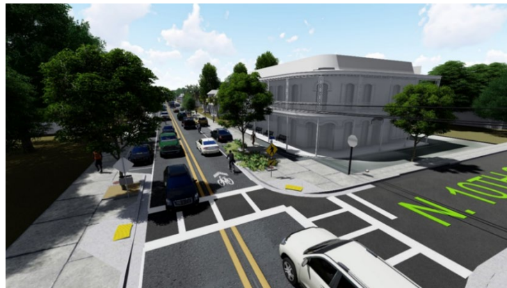
Figure 2 - Visualization of E Columbus Dr with Proposed Improvements near North 10 th St displaying cross walks, share-the-road bicycle markings, on street parking, corner bulbouts and curb ramps.
