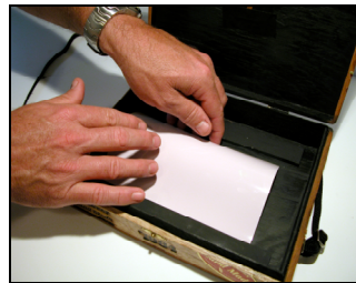
Photo 3, 4 and 5. Loading the cigar box pinhole camera.
