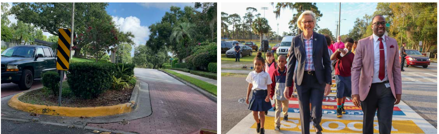
Traffic calming devices such as narrowed lanes, speed humps, and particularly planted islands and circles significantly slow neighborhood vehicles speeding, particularly on long block segments. The City of Tampa's FDOT award-winning "Crosswalks to Classrooms" program demonstrates the power of street graphics to provide clearly marked, visually impactful routes for children and motorists to view and helps to brand the neighborhood "Safe Routes to Schools".
