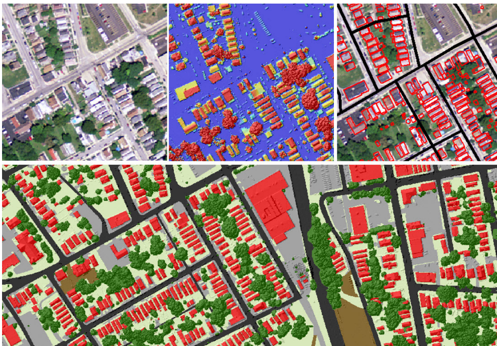
Figure 5. Aerial images, LiDAR and ancillary map data are used to create the detailed land cover maps.
