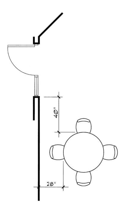
Any table located adjacent to an exit must be placed so the edge of the table is no less than 40 inches from the exit discharge. The exit discharge will include the width of the door, and alcove or recess, or any other portion of the exit. Any table located adjacent to a fire department sprinkler connection (not shown). Must be placed so the edge of the table is 55 inches from the edge of the FDC.
