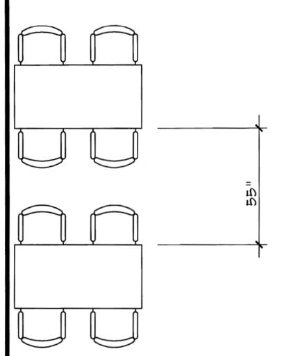
Where square or rectangular tables are arranged parallel to each other and perpendicular to the wall, there shall be at least 55 inches between tables. There is no minimum distance between the tables and the wall. The tables may be against the wall.
