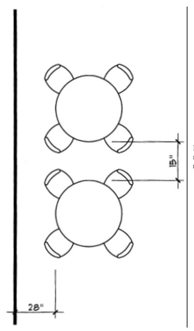
If the chair locations are rotated as shown, the distance between tables may be reduced to 15 inches. The distance between table to wall shall remain 28 inches.
