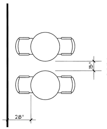
When tables are arranged side by side, with no chairs arranged between the tables, there shall be no less than 15 inches between the tables. There shall be no less than 28 inches between the tables and a wall or other obstruction.
