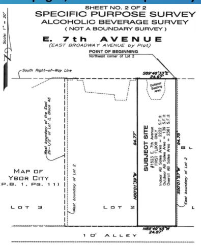
BASIS OF BEARINGS: For the purposes of this survey the South right-of-way line of East 7th Avenue has an assumed bearing of N.89'46'33"E.)
