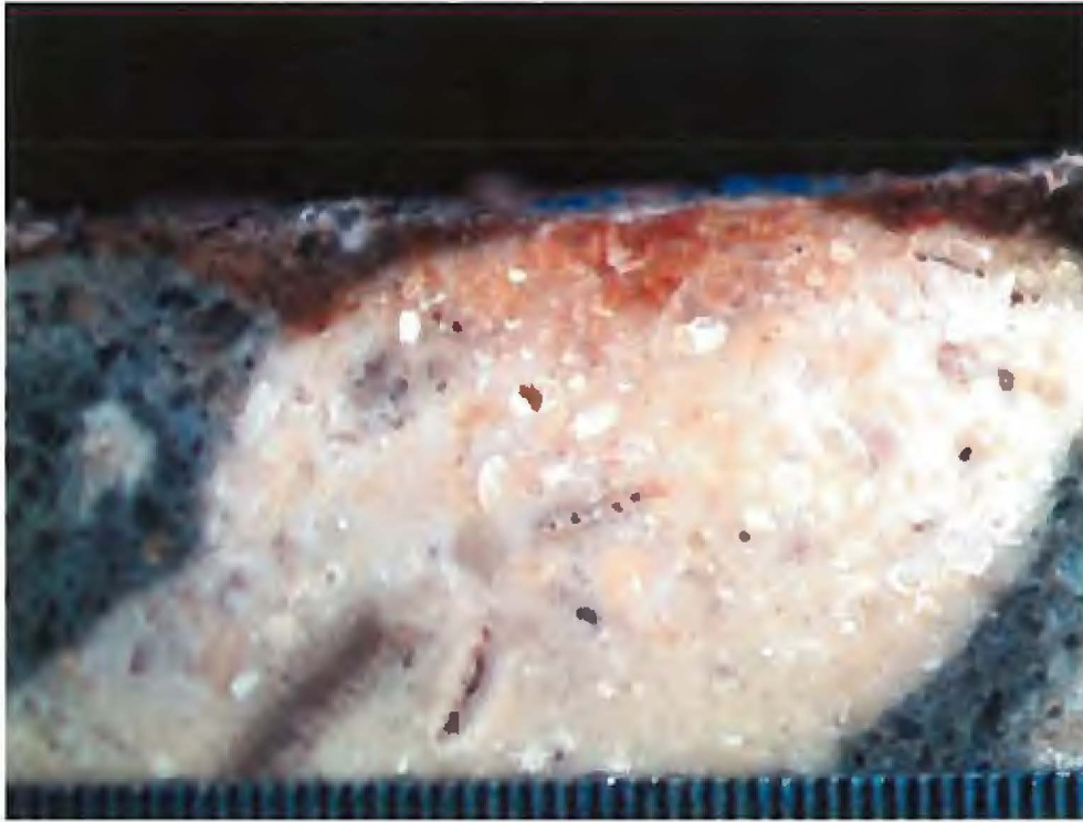
Photo 6 – Magnified view of stain inclusion (Struvite) getting deeper at coarse aggregate piece. Scale = 0.01 inches
