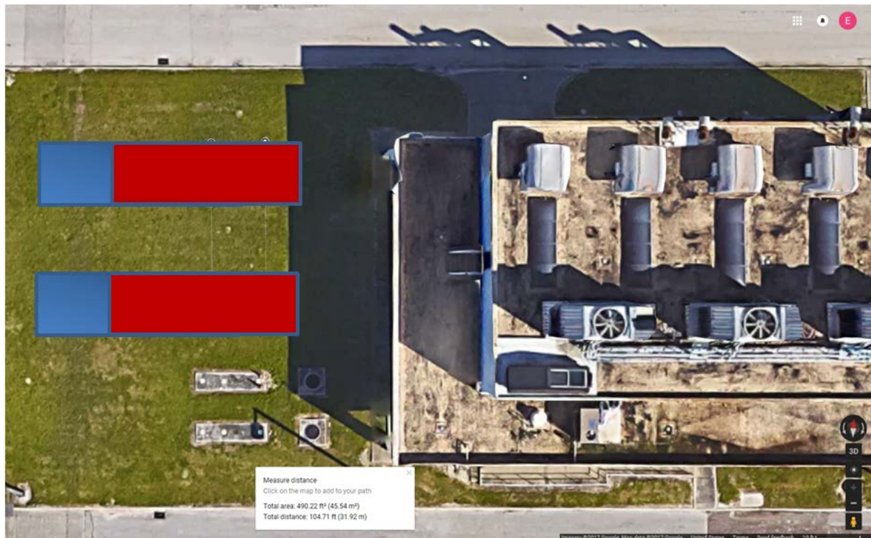
Figure ES.2-10: Footprint of Aboveground Fuel Storage Tanks
