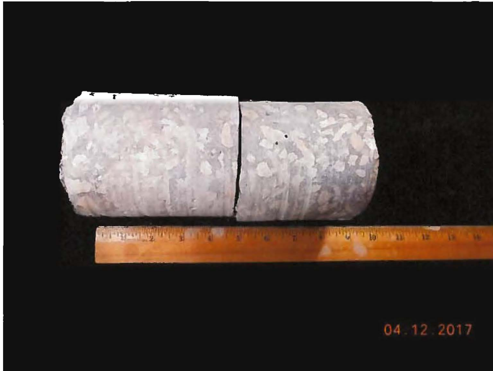
Photo 1 – Sample C-05 (sample cut to allow insertion into saw for longitudinal cut)
