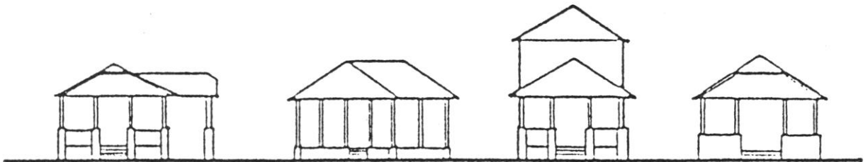
Appropriate: porch and hipped roof break down height and mass of building.
