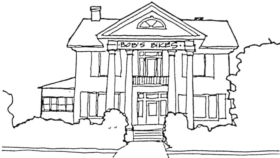
Inappropriate: Wall sign is too large and obscures architectural detail.
