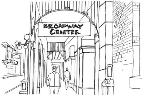
Projecting sign hung in archway
