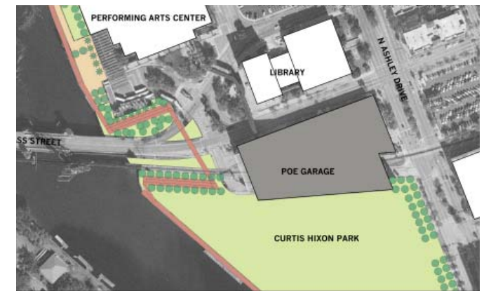
Figure 3.19 Option 3 – Cass/CSX Bridge: over bridge switchback ramp system.
