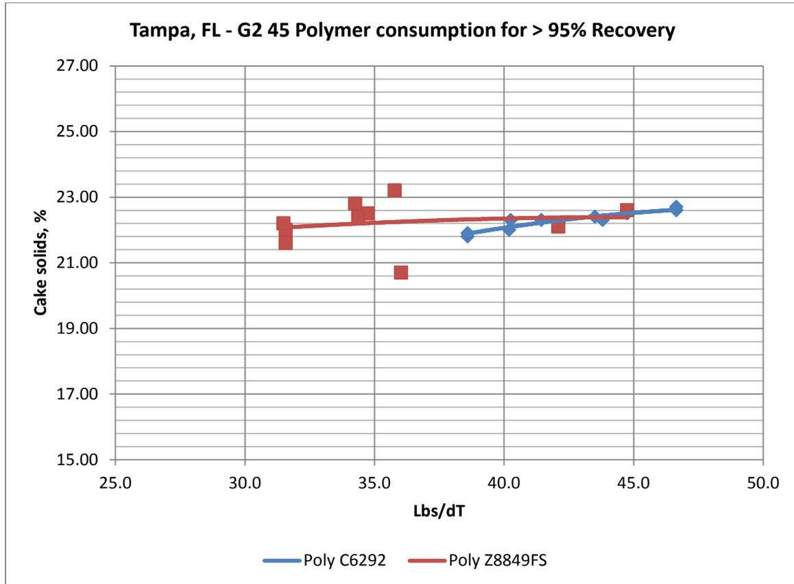
The polymer consumption is deemed to be in the high side for this type of sludge. It is possible that changing the conditions at the process in the plant would reflect in a much more economical dewatering operation.
