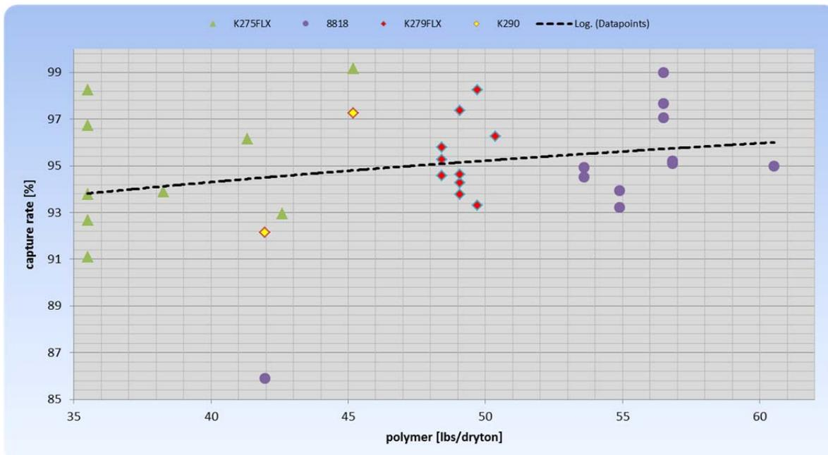
As shown in Figure 8, the capture rate improved with increasing polymer consumption. The first few data points show a lower capture rate which is typical during the initial press setup. Once the optimal settings are determined, consistently high results can be expected. The capture rate was 93% or better when the polymer consumption rate was between 47 and 57 lbs active/ton DS. The K279 FLX and the 8818 polymere provided the best overall performance and capture rate.
