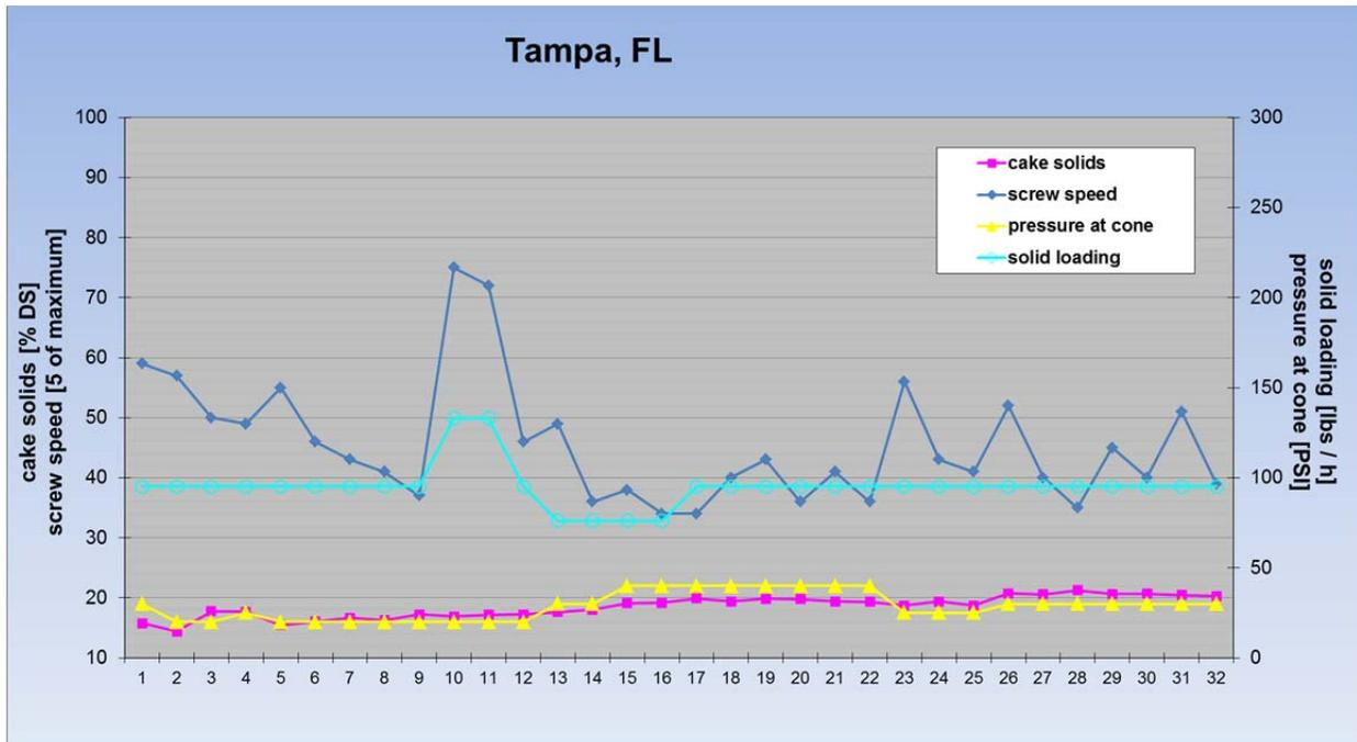
The cake solids consistently ranged between 18% and 21% DS. The polymer consumption was maintained within a range of 34.5 and 60.5 lbs. active / ton DS to ensure good dewatering performance.
