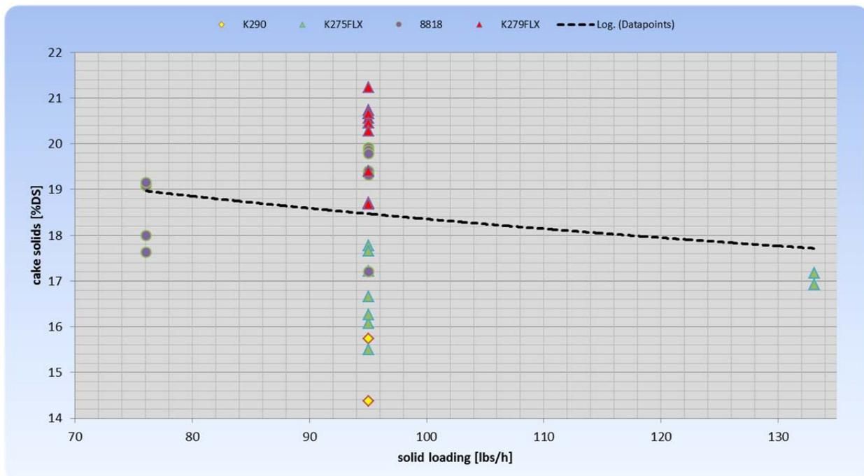
In general the effect of the solids loading on the discharged cake solids is also related to the screw speed. The solids loading determines the speed of the auger with higher loading rates requiring higher screw speeds which can often result in a lower discharging rate of cake solids.
