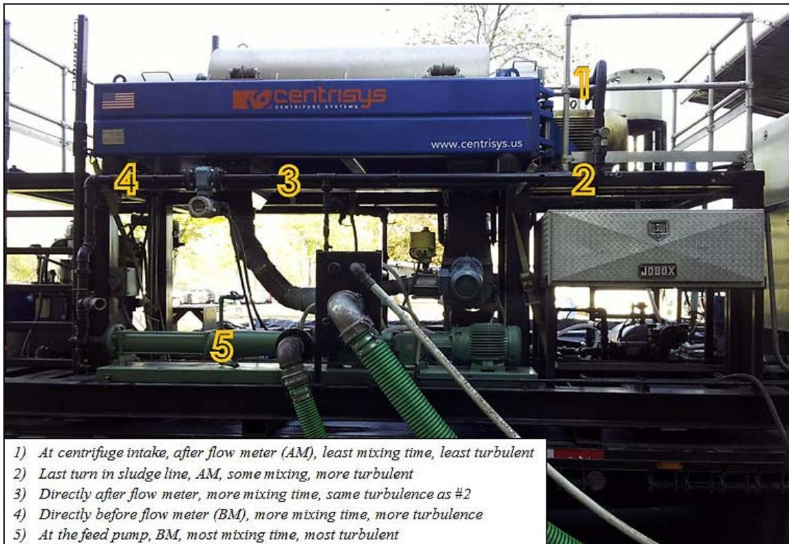
Figure 2: Various polymer injection points
