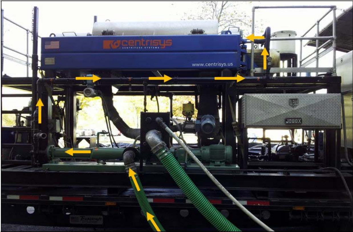
Figure3: Sludge Feed Flow
