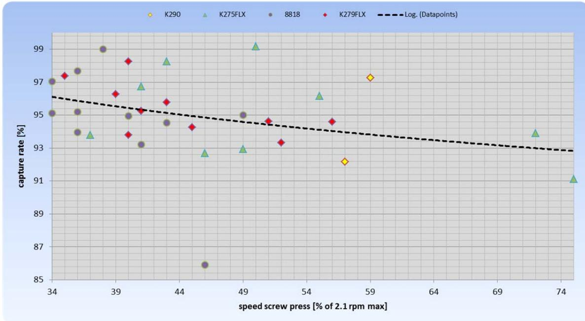
The test results in Figure 9 above show a variation in capture rate which is typically highly affected by the screw press speed. The capture rate drops gradually when operating the screw press with speeds ranging from 34% to 75% of its maximum 2.1 rpm.
