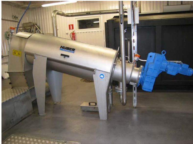
cleaned with spray water from the outside. The screw stops and reverses rotating the basket through 360° allowing the spray bar to fully wash the exterior surface of the basket within the enclosure. The screw pushes dewatered sludge to the upper end of the basket where it compressed against a pressure cone maximizing dewatering performance before discharging and dropping down a chute into a dumpster.
