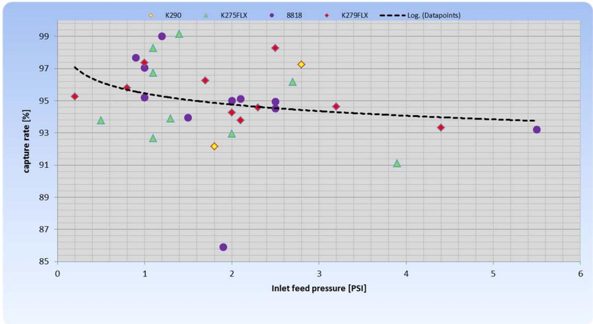
The pressure at the inlet flange applied to the feed also has a significant effect on the capture rate as shown in Figure 10 above. The pressure ratings exceeding approximately 2.5 psi caused the capture rate to decrease below an acceptable level.
