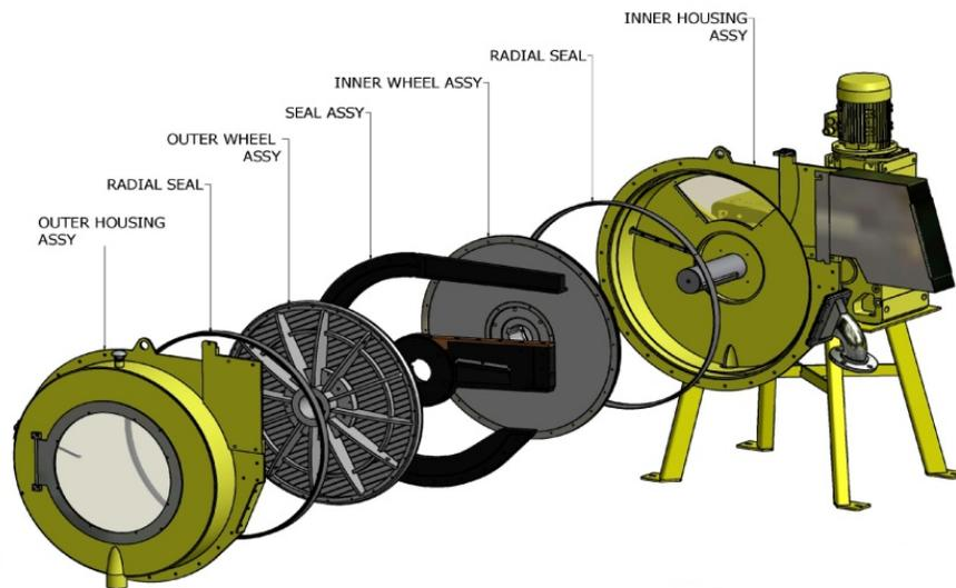
**Figure 1 – Basic Construction of the Prime Solution Rotary Fan Press®**
