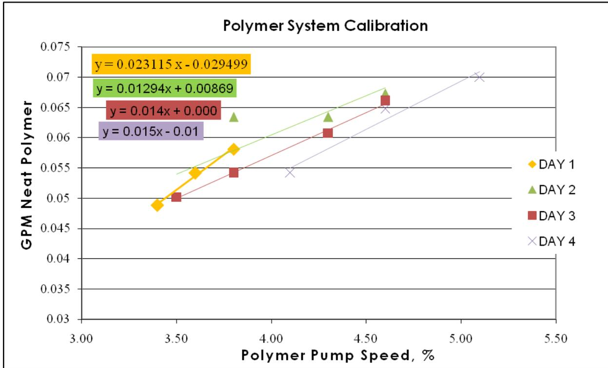
Figure 1: Daily Polymer Pump Dose Calibration
