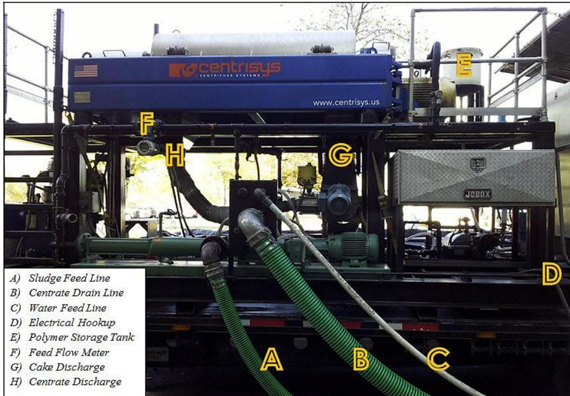
Figure 1: Key components of the pilot test trailer
