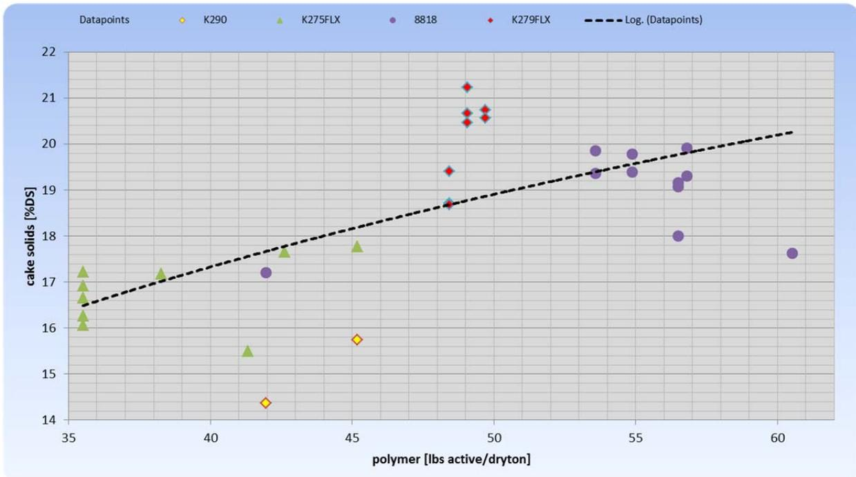
The cake solids are consistent between 18% and 21% when using 48 – 57 lbs. active / ton DS. The excessive use of polymer above 57 lbs. active / ton DS is of no benefit.
