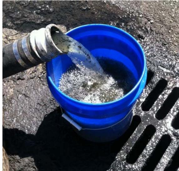
Photo 4: Pressate from Screw Press
