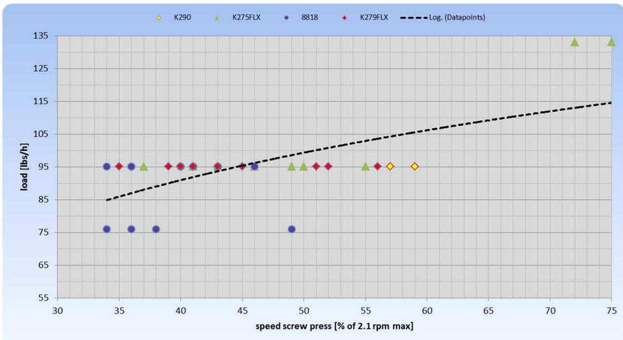
This point of operation changes with many parameters: polymer dosing, polymer injection and mixing system, hydraulic and solids loading, screw speed, and cone pressure. It is a very complex relationship and very sensitive to fluctuations. For peak efficiency and performance the screw press should be operated just below the point that it is overloaded.
