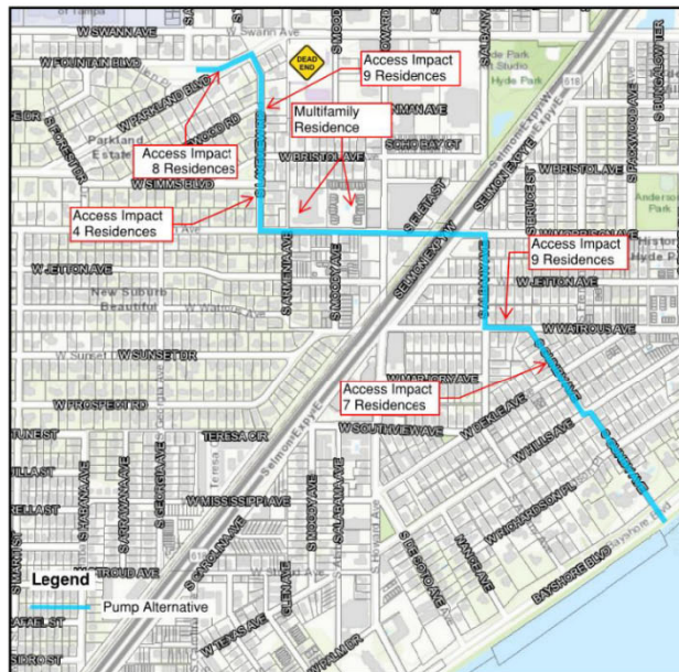
FIGURE 14. Pump Alternative Impacts to Access
