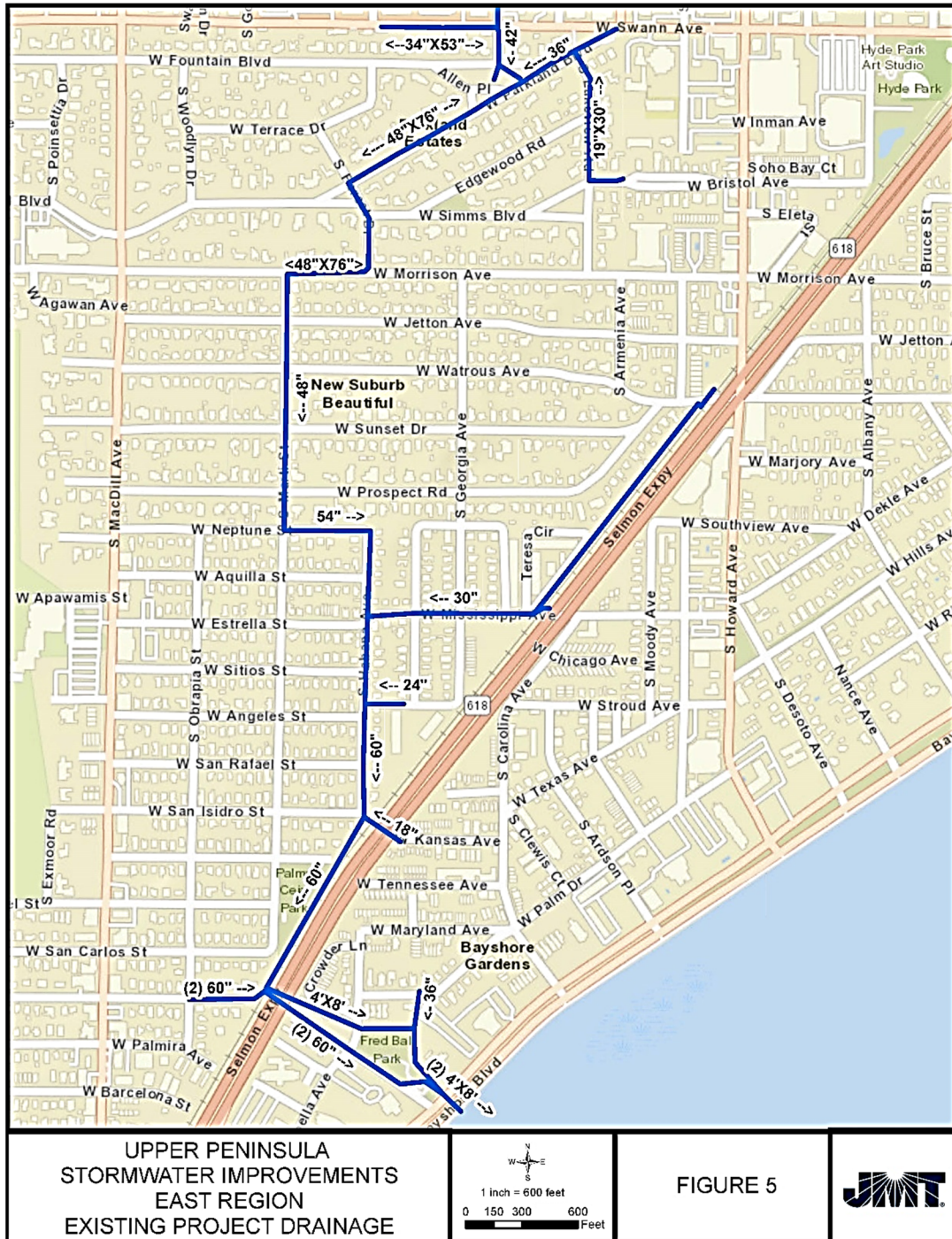
Figure 5: Existing Drainage Network
