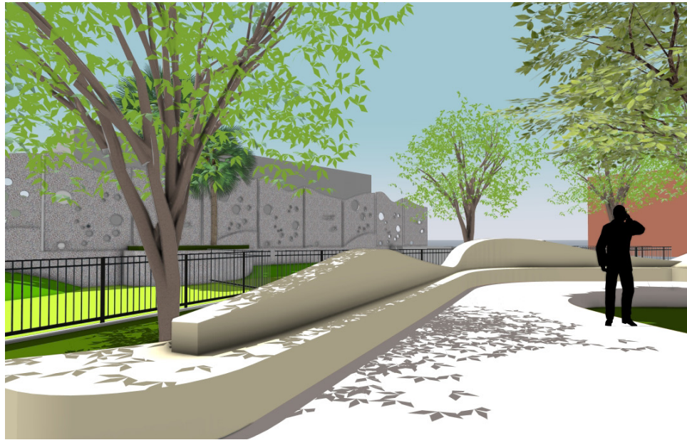
PRECAST SEAT WALL WITH BACK
