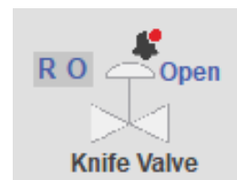
Figure 32 Knife valve alarm
