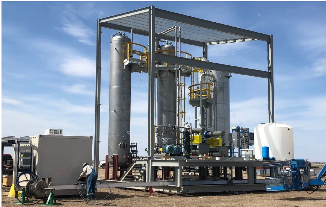
Figure 3-4: Catalytic-Caustic Scrubbing System (SULFCAT)
