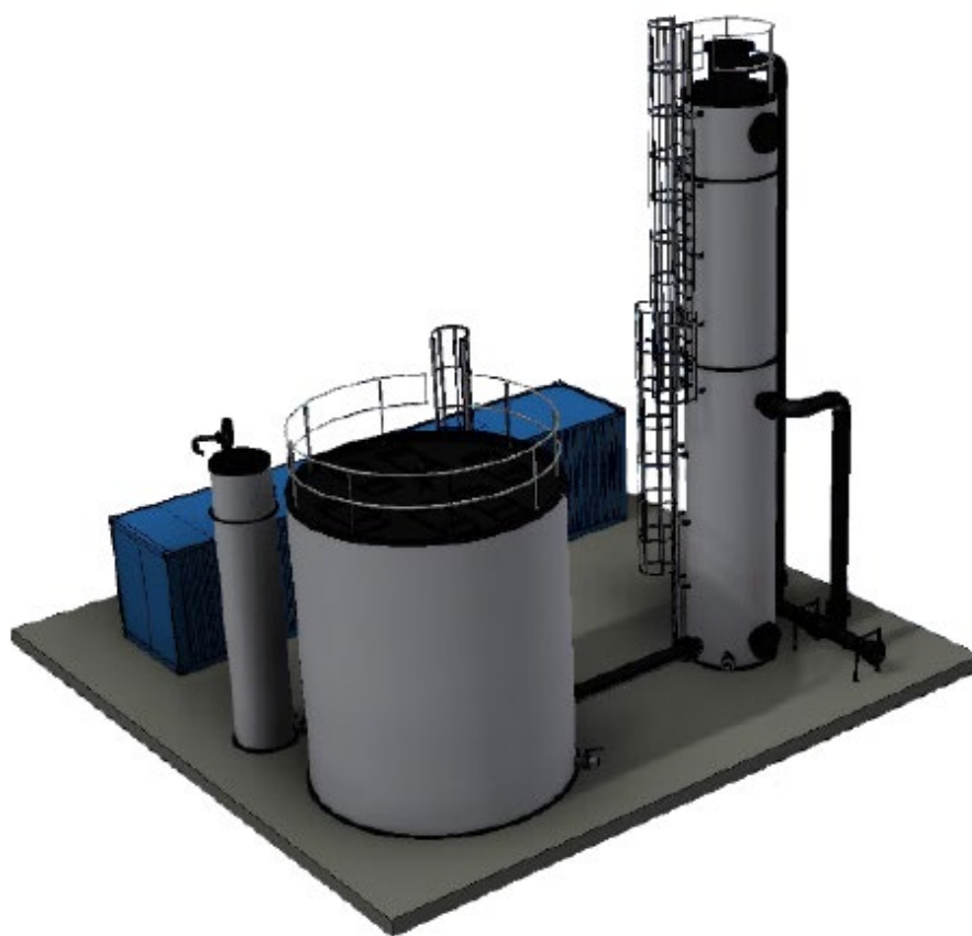
Figure 3-3: Bio-Caustic Scrubbing System (DMT)
