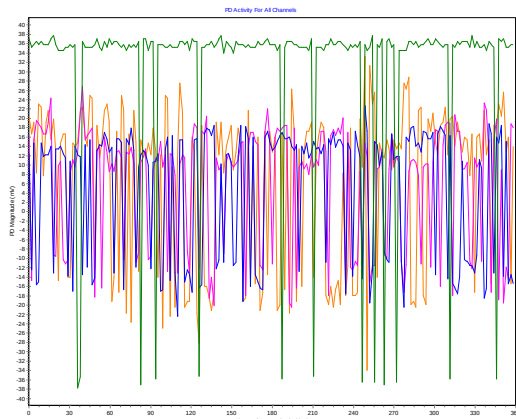
Phase-Resolved Graph (PD and Noise)
