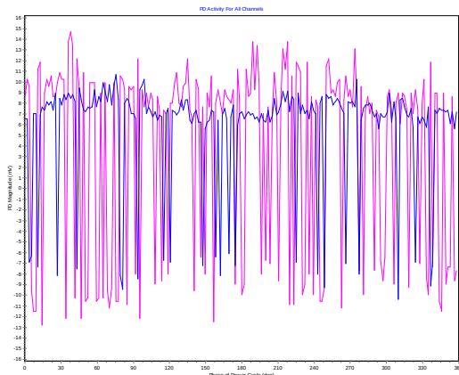
Phase-Resolved Graph (PD and Noise)
