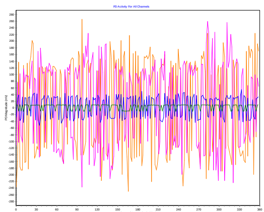
Phase-Resolved Graph (PD and Noise)
