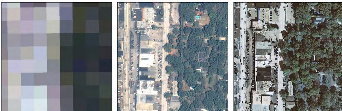
Figure 23. Resolution of imagery used for long-term trend (Landsat), 2006 analysis and 2011 analysis, from left to right.
